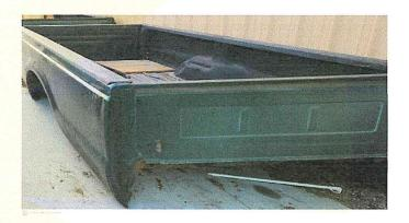
2. Pickup box removed for installation for flatbed conversions
